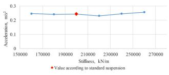
Fig. 8. Dependence of mean square of carbody accelerations on the lateral stiffness of the secondary suspensionsuspension
