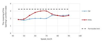
Fig. 4. Sperling's comfort index values in the lateral direction in 200 m radius curve
