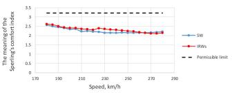
Fig. 10. The value of the Sperling's comfort index in the vertical direction in tangent track
